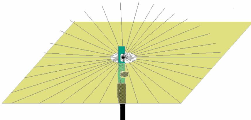
Fig. 4: Illustration of omni-directional XS sensor head.
