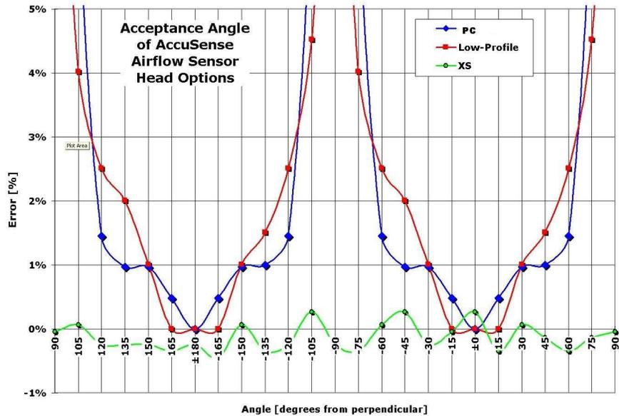
Fig. 2: Accuracy of AccuSense sensors vs. angle from perpendicular of oncoming airflow.
