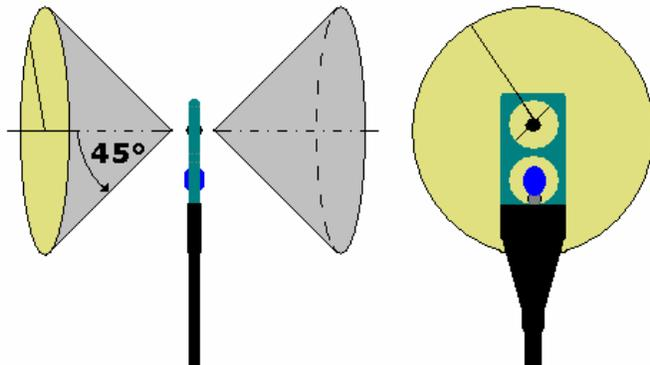
Fig. 3: Airflow acceptance angle for PC and Low-Profile sensor heads as recommended by AccuSense.
