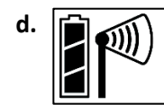
Once the mote has finished joining the network, the "x" icon is removed and the channel count on the station LCD increases by three (two for water potential and temperature, and one for the mote battery).
