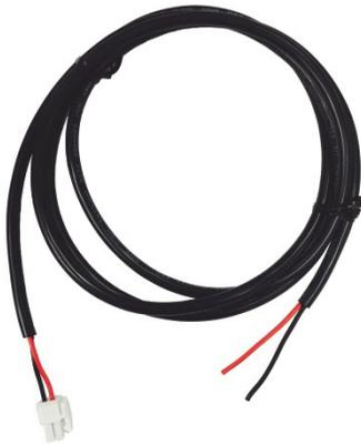
The external DC power cable (CABLE-RX-PWR) is used to connect a user-supplied power source to the HOB0 RX3000 Monitoring Station to charge the station's internal battery. The external power source can be an intermittent power source, such as a 6W or larger solar panel. The external power source must be able to supply 6W, but the average power used will be much less and depends on the number and type of sensors, logging interval, and the frequency of internet connections.
