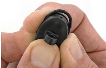
5. Inspect the O-ring for cracks or cuts and replace it if any are detected (the O-ring is included in the Pendant replacement parts kit, UA-PARTSKIT).
