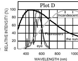
The StowAway LI logger is calibrated on an incandescent source, and will read about a factor of twelve low for fluorescent lighting, and about a factor of six low when measuring indirect sunlight.
