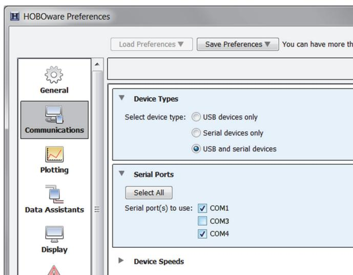
Click OK in the Preferences window to save these settings. HOBOware should now be configured to work with the Keyspan USB-to-serial adapter.
