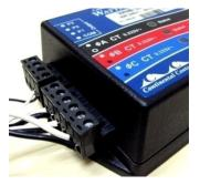
6. Connect Voltage Input Lead Set to the Screw Terminal Block on the WattNode.
