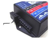
5. Connect Current Transducer(s) to the CT Block on the WattNode.
