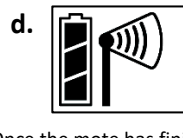
Once the mote has finished joining the network, the X icon disappears and the channel count on the station LCD increases by three (two for soil moisture and temperature, and one for the mote battery).
