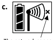
The network connection X icon blinks while the mote completes the registration process, which may take up to five minutes.
