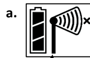
The signal strength icon blinks while the mote is searching for a network.
