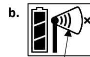
Once the mote finds a network, the icon stops flashing and the bars cycle from left to right.
