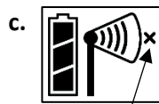
The network connection X icon blinks while the mote completes the registration process, which may take up to five minutes.
