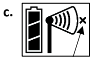
The network connection X icon blinks while the repeater completes the registration process, which may take up to five minutes.
