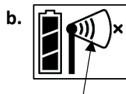
Once the repeater finds a network, the icon stops flashing and the bars cycle from left to right.
