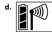
Once the mote has finished joining the network, the X icon disappears and the channel count on the station LCD increases by two (one for rainfall and one for the mote battery).
