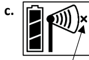
The network connection X icon blinks while the mote completes the registration process, which may take up to five minutes.
