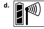
Once the mote has finished joining the network, the X icon disappears and the channel count on the station LCD increases by two (one for temperature and one for the mote battery).
