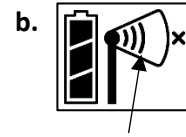
Once the mote finds a network, the icon stops flashing and the bars cycle from left to right.
