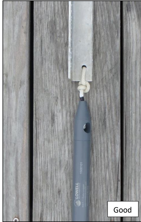
Figure 2A (top left): The recommended mounting method for an aluminum bracket is to drill through the bracket, deburr the hole and knot on the back side.
