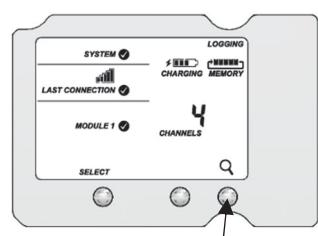
Press the Search button. The magnifying glass icon blinks while the station is in search mode waiting for repeaters to join the network.
