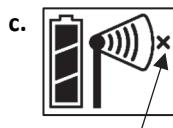
The network connection "x" icon blinks while the repeater completes the registration process, which may take up to five minutes.
