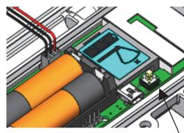
Open the repeater door and install the rechargeable batteries. Press this button on the repeater for 3 seconds.
