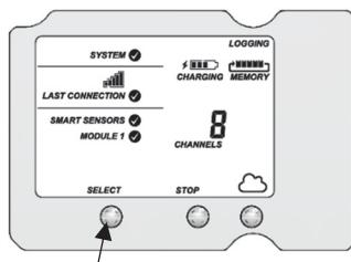
Press the Select button on the station to switch to the module with the manager (module 2 on RX2105 or RX2106 stations).
