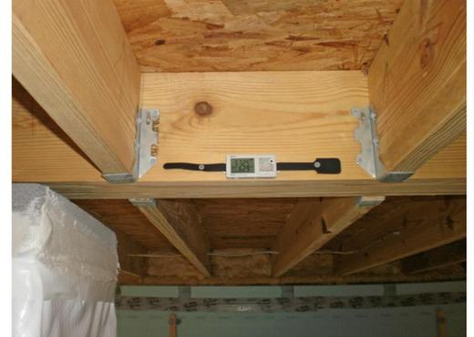
The compact, affordable HOBO UX100 temperature data loggers, which feature an easy-to-view LCD display and large memory capacity, were deployed in crawl spaces and attics of both houses to measure and record temperature and relative humidity around the clock over the next year. Data from the loggers will be analyzed and used to prove energy-efficiency gains realized with new green building and energy-efficient construction techniques.
