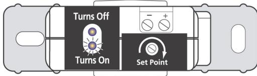
STEP 1: Turn the setpoint screw clockwise until the Status Closed LED turns off and the Status Open LED turns on.
