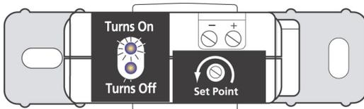
STEP 1: Turn the setpoint screw counter-clockwise until the Status Open LED turns off and the Status Closed LED turns on. (Sensor should be in this state right out of the box.)
