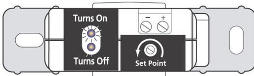
STEP 2: Slowly turn the setpoint screw counter-clockwise until the Status Closed LED turns on and the Status Open LED turns off.
