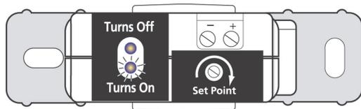
STEP 2: Slowly turn the setpoint screw clockwise until the Status Closed LED turns off and the Status Open LED turns on.
