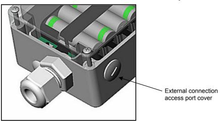
2. Insert the cable through the external connection access port. Screw in the fitting to seal the hole. Hand-tighten the fitting and then tighten an additional ½ to ¾ turn with a crescent wrench.
