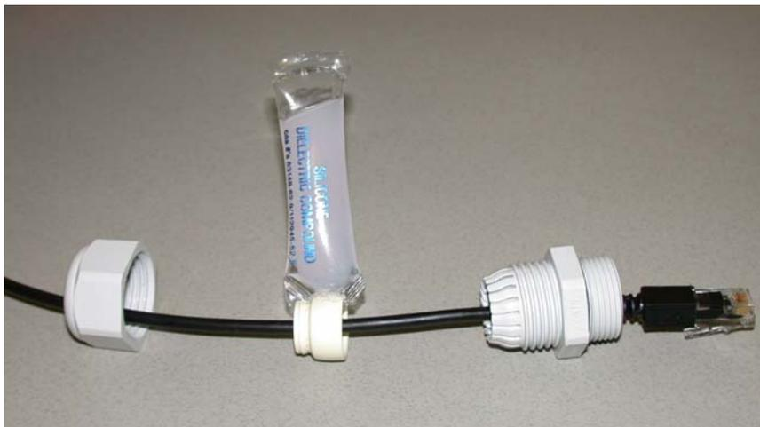
6. Push the slit insert back into the PG-16 body and slide the cable up so that the plug can be moved aside. Pushing the slit insert in at a slight angle and with a slight twist may help it slide in more smoothly.
