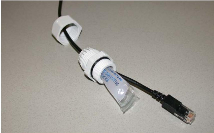
8. Plug the cable into the coupler included with the extension cable.
