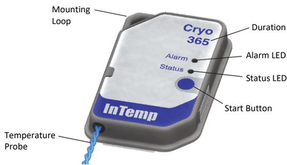
**Mounting Loop:** Use this to tie the logger to the materials being monitored.
