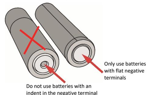
To install or replace the batteries:
