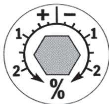
Moving the screws in the positive (+) direction causes the spoons to tip more times (i.e. give a larger count) for a given amount of water. Modify both adjustment screws by the same amount.
