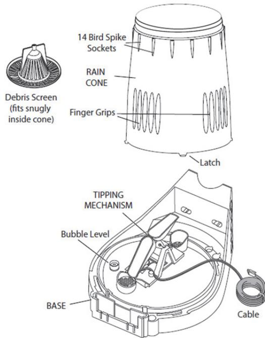
These are the internal components on the base in more detail.
