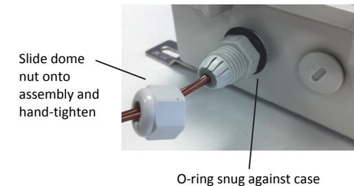
3. Repeat steps 6 and 7 with the other assembly and thermocouples. If there are no thermocouples in the other port, then screw the dome plug into the open port so the O-ring is snug against the case as shown below.
