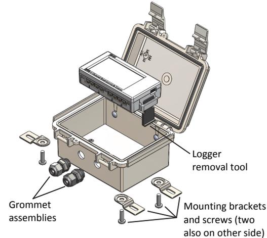
1. Use a Phillips screwdriver to attach the four mounting brackets to the back of the case.
