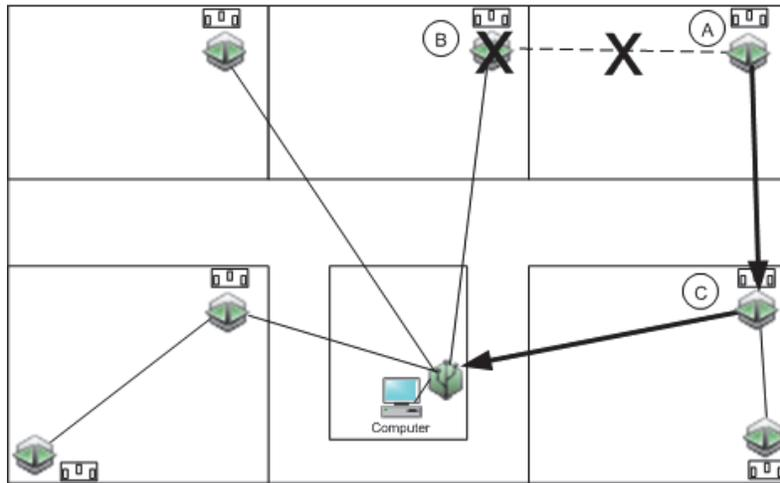
Figure 8: Automatic Rerouting
