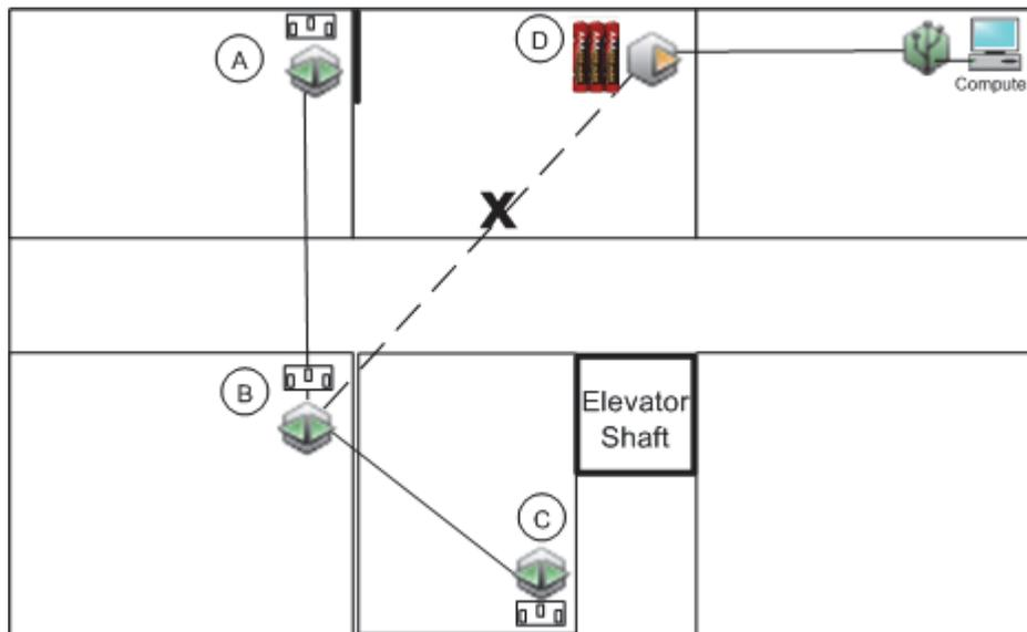
Figure 9: No Routing on a Data Node
