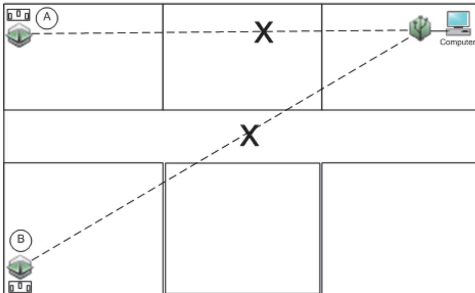
Figure 4: Data Nodes Cannot Connect to the Receiver
