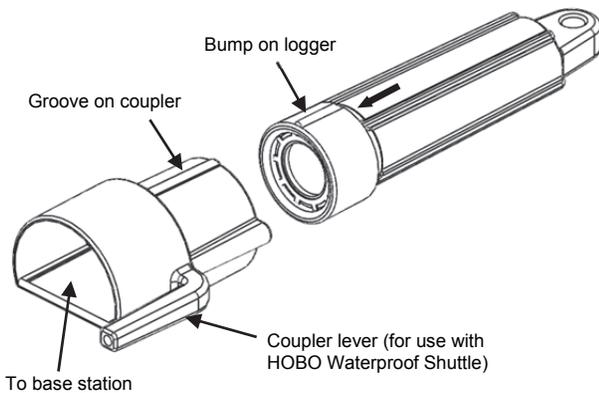
If you are using an older model of this logger and the arrow is not visible, hold the curved side of the coupler up as shown above. Insert the logger with the flat side up (the side in line with the flat side of the mounting hole).
