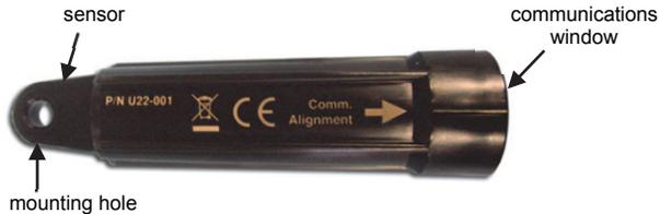
**Important:** The plastic case will become brittle at temperatures lower than  $-20^{\circ}\text{C}$ . If the logger is deployed in a location where the temperature drops below  $-20^{\circ}\text{C}$ , make sure the logger remains stationary and is not pulled on or struck. Return the logger to above  $-20^{\circ}\text{C}$  before handling.
