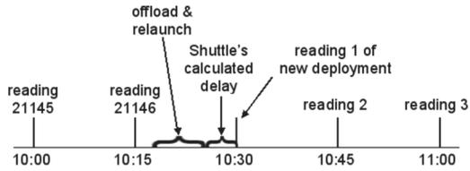
**Important:** If the logger was launched with multiple logging intervals, there will be no synchronizing delay. The logger will start immediately with the last defined logging interval.
