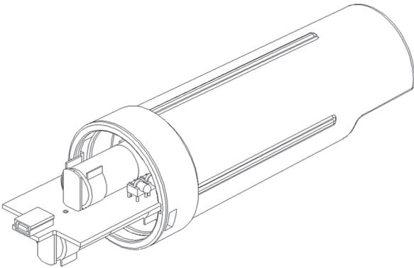
6. Remove the old batteries and install two new ones in the correct orientation. Both batteries should be turned the same way, with their positive ends facing the USB port on the board. (When the second battery makes contact, all of the shuttle's LEDs will blink in unison.) It is recommended that you replace the desiccant (DESICCANT2) when replacing the batteries.
