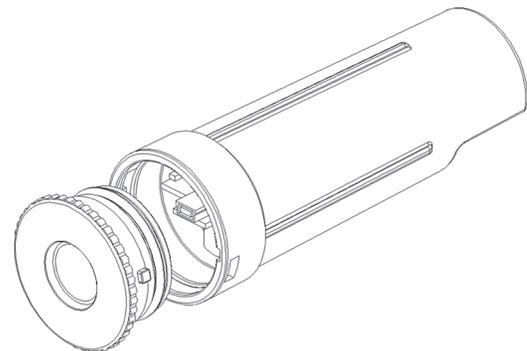
5. Turn the shuttle over and tap it gently. The circuit board should slide into your hand.
