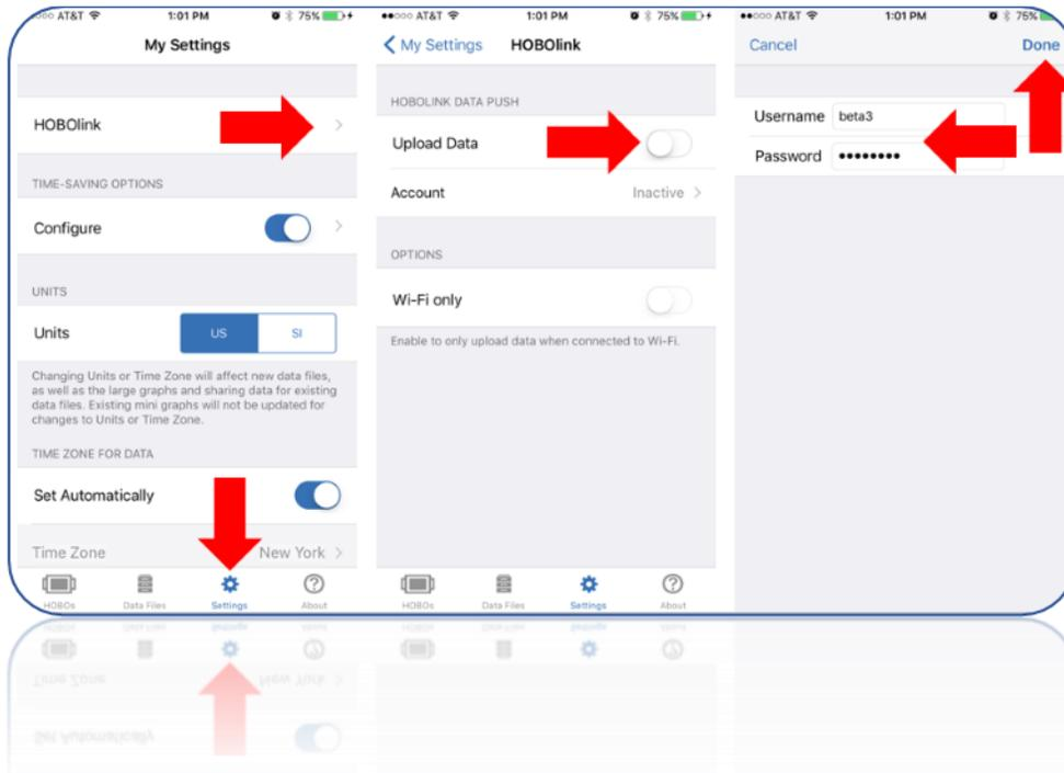
Step 3. Now, when you connect and readout an MX data logger, the data will be uploaded to your HOBOLink account. You can stop here if you are only using HOBOLink for addition safe data storage.
