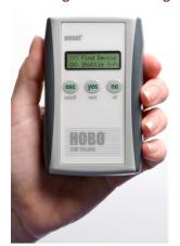
Take readings every step of the installation with a HOBO Shuttle or HOBOware. This can help you identify potential air gaps, compaction issues, and even severed cables. This is highly recommended for any large installation.
