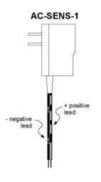
Polarity is very important - there is a bold white (broken) stripe marking the positive lead. The negative lead has no stripe and only has tiny lettering.
