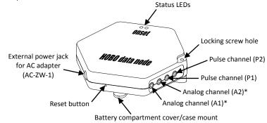
\*Caution: Analog channel input cannot exceed 2.5 VDC. For sensor outputs up to 10 VDC, use appropriate voltage adapter cable.
