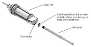
After installing the antenna, connect the HOBOnode Outdoor Receiver to the PC. Put the receiver into the base and mount vertically or lay horizontally on a desk. Make sure the antenna is pointing upward. The receiver will automatically connect to HOBOnode Viewer within approximately 1 to 2 minutes and an icon will appear in the Network Tree. Only one HOBOnode Outdoor Receiver can be connected to a single PC.
