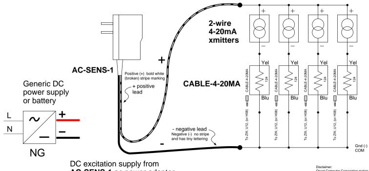
AC-SENS-1 ac power adapter shown, generic OK also. http://www.onsetcomp.com/products/adapters/ac-sens-1
