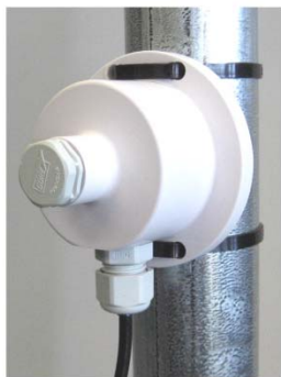
Figure 1: S-BPB Mounted to Tripod Mast
